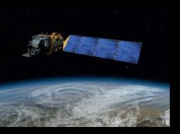
sat 8's data is displayed in the visible spectrum (i.e. what we can see), it also maps vital non-visible information that, when rendered using special imaging techniques, can reveal geological properties, such as hidden mineral deposits.
